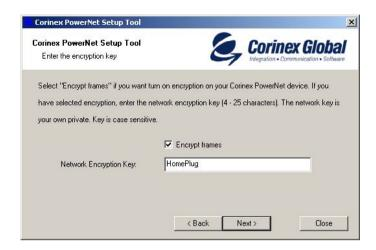
• Click 'Next' again to program the Corinex Intelligent PowerNet Ethernet Adapter with the new encryption key. This will take a few seconds. The next screen will look similar to the following screen. The white box will list the MAC addresses of all other installed powerline devices on the network that are programmed with your chosen network password. If no other devices have been programmed, the list will be empty.
